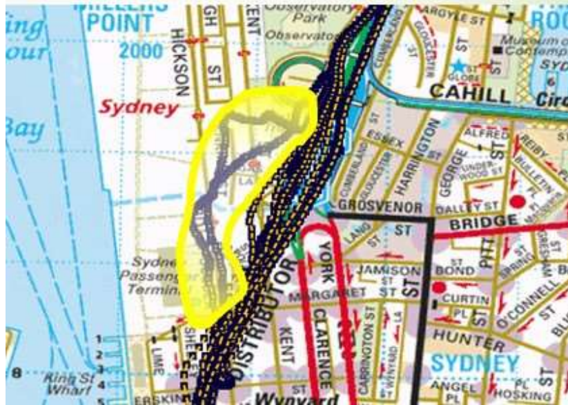
Figure 8 - is of the road network immediately south of the Harbour Bridge in Sydney. There are two trips (highlighted with a yellow boundary) that appear to have deviated from the defined route. The recording was from a survey vehicle that we knew did not take this path off the digitised road network nor through buildings.
