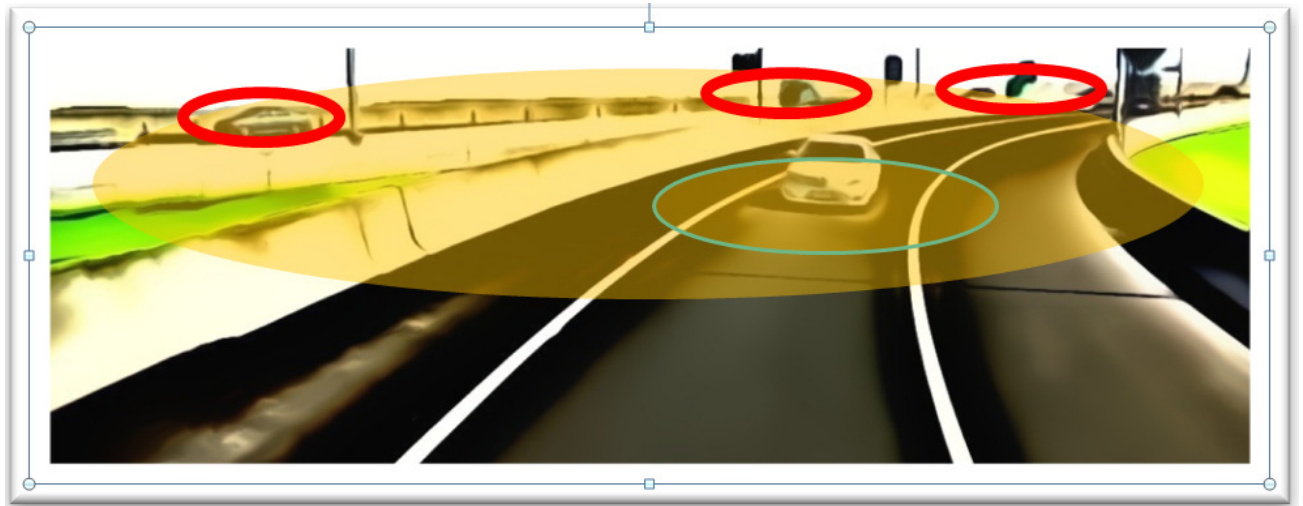
Figure 2 Extraneous sensed probes (Red) not in the corridor of interest (Green), Report by Scott Benjamin then Austraffic now WSP
